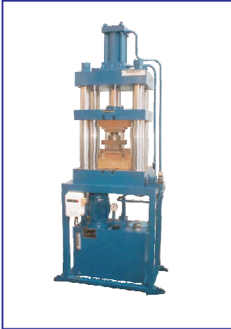
50T, 4 pillar type, moving platen hydraulic press for gasket forming.
